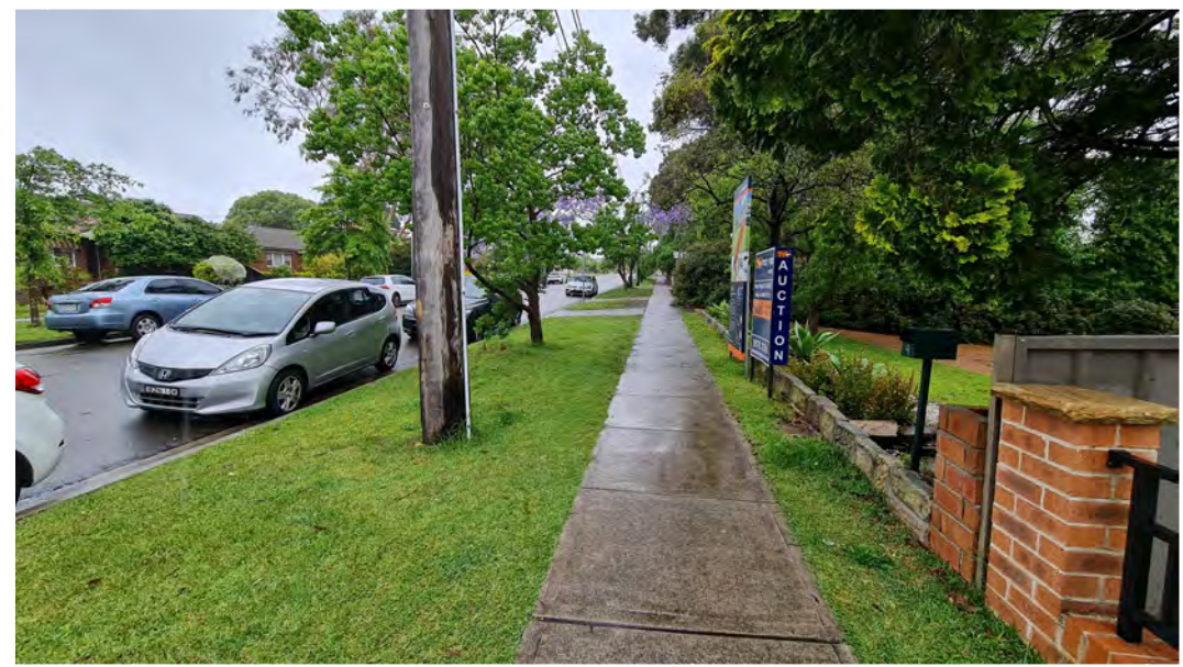
PHOTO 01: LINCOLN STREET FRONTAGE. EXISTING COUNCIL VERGE, FOOTPATH, UTILITY POLE AND STREET TREE. EXISTING SITE VFC AND DRIVEWAY. PROPOSED VFC AND DRIVEWAY AMENDMENT(WIDEN AND RENEW) TO FUTURE CIVIL DETAIL, ALL OTHER ITEMS RETAINED / RESTORED / PROTECTED.
