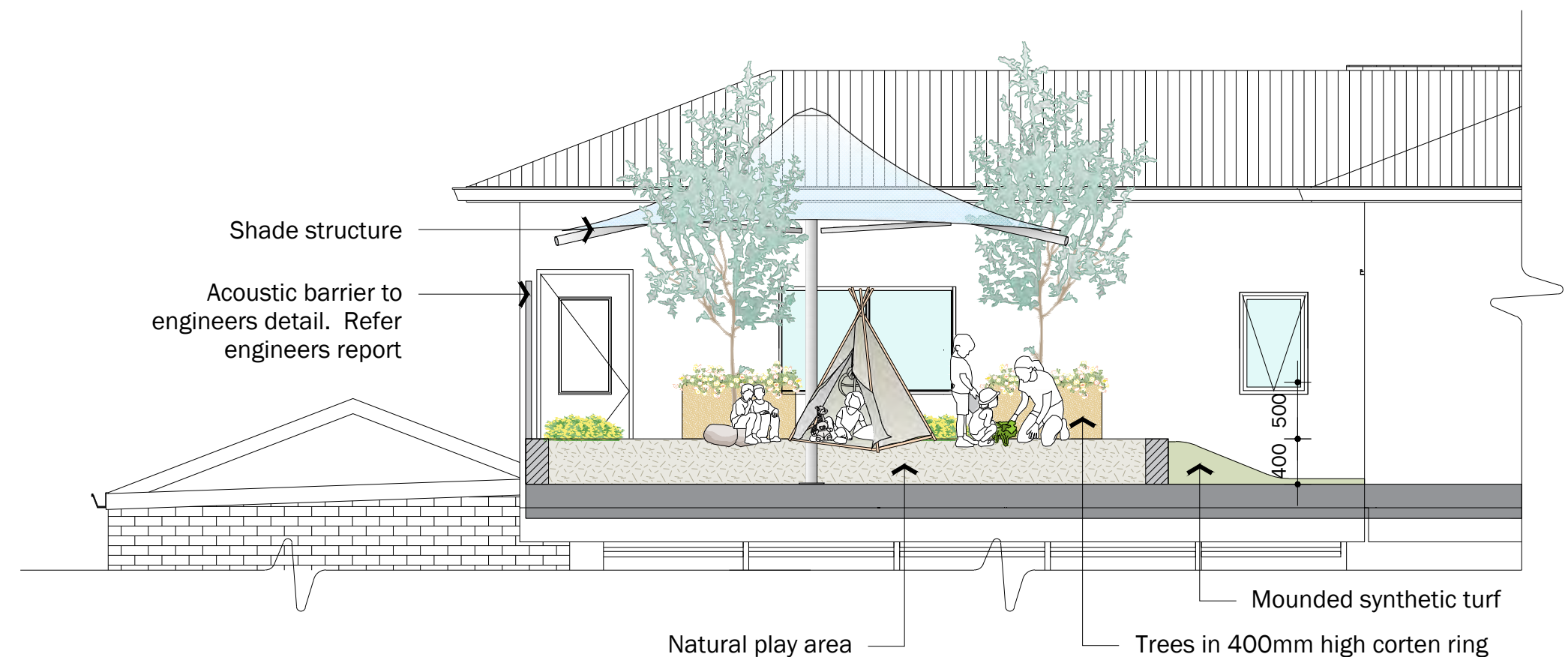
04 TREES ON STRUCTURE TYPICAL DETAIL All structures and grades to engineers details 1:50
