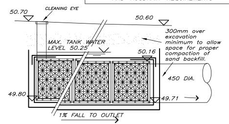
TANK MODULES WRAPPED IN GEO-TEXTILE FABRIC. BASE AND SIDES TO BE LINED FIRST WITH POLYPROPYLENE PLASTIC TO PROTECT GEO-FABRIC
