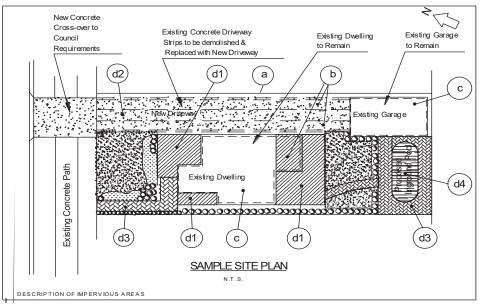
**Post-development impervious area**: This includes all of the impervious areas within the site which are to remain after the development is completed, that is, the finished works, and includes all of the *retained, existing* and *proposed impervious area*.
